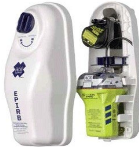
Figure 10. ACR 2842 Cat 1 406MHz EPIRB that was reportedly carried onboard the CONCH'RD at the time of the sinking.
